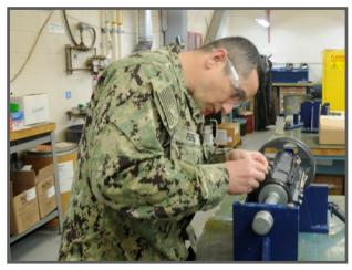
FC1 (SW/AW) Alexander Perez lockwiring remover track spacers on a CIWS gun rotor.
