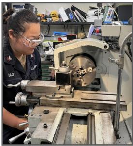
MR2 Yingli Cao uses the lathe aboard USS John Finn (DDG 113) to manufacture a shear pin to fix a lathe.
