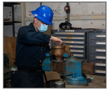
A USS Dwight D. Eisenhower (CVN 69) Sailor disassembles a relief valve while on board the NNSY Valve Barge. The Valve Barge has been in operation for over 20 years and is capable of overhauling and testing a wide variety of valves used on Navy assets. (Photo by NNSY Photographer, Mrs. Shelby West.)
