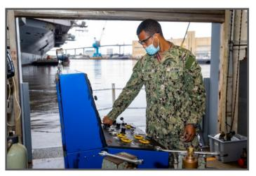
A Sailor on the NNSY Valve Barge operates a test stand to hydro test relief valves. (Photo by NNSY Photographer, Mrs. Shelby West.)
