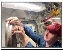
DC3(SW) Nathan Harris con-ducting a permanent set/ groove measurement in the MAFO-Holtkamp door gasket with DC1(SW) Jonson Frais observing. (Photo by Ramir Pulido.)
