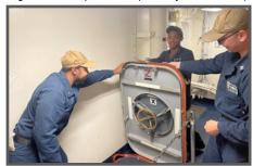
L-R: MR3 Jordan Point being assisted by Divisional Damage Control Petty Officers EN3 Courtney Davis and FC2(SW) Steven in safely placing Watertight Hatch in a safe maintenance position in order to properly conduct a gasket channel inspection and gasket replacement. (Photo by Ramir Pulido.)
