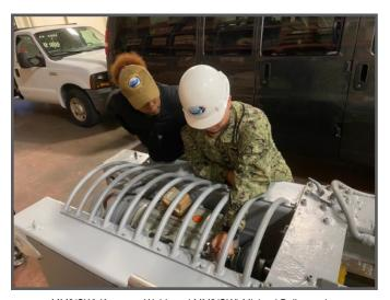
MM2(SW) Kareema Webb and MM2(SW) Michael Bailey make adjustments to the flexible coupling on a sliding pad-eye off USS Stout (DDG-55). The flexible couple is used to absorb a slight misalignment with the main electrical motor and the ball screw. (Photo by MM2(SW) Jonathan Lepley.)
