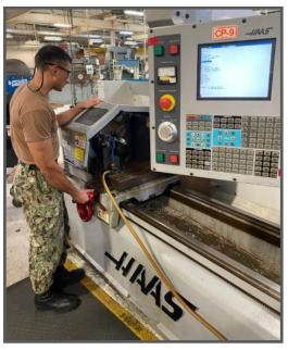
NAMTS Sailor, MR2(SW) John Suarez, positions the CNC Lathe cutting tool into home position before activation of the CNC machining process of a deck plug at Southeast Regional Maintenance Center (SERMC) Code 941, Inside Machine Shop. (Photo by Rick Smith.)
