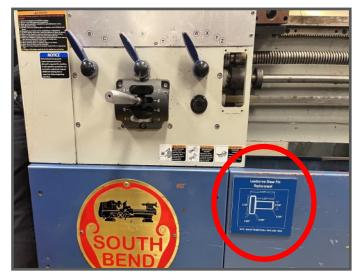
MR2 Yingli Cao created a drawing on the engraving machine, produced it and placed it on the lathe's bed, right below the opening where the shear pin is located.
