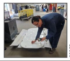
Liz Curiel measures final paint thickness using a handheld ultrasonic tester. (Photo by Doug Scholl.)
