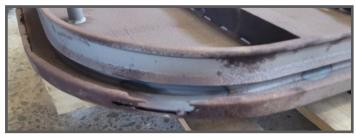
A corroded watertight door is kept in the shop as a sample of sever degradation. (Photo by Doug Scholl.)
