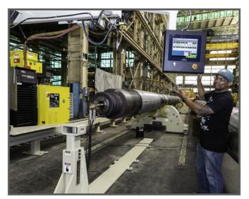
Welding Supervisor Donovan Harris shows how to use the control panel for the newly acquired Computer Numerical Controlled (CNC) Submerged Arc Welder (SAW) at Norfolk Naval Shipyard on July 12, 2021. (Photo by Aldo Anderson.)
