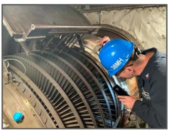
GSM2 Schillinger is conducting a Gas Turbine Bulletin 12 inspection on a Turbine.
