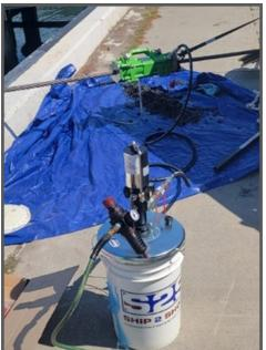
Ship2Shore, Inc. The aforementioned VI-PER is a device that is clamped onto the extended cable and held in position by securing straps while the cable is retracted back into the craft. It removes the old grease and debris from the cable then penetrates the cleaned cable with Military Standards (MIL-STD) approved lubricant.
