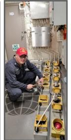
While EM2 Oscar Alfaro is conducting repairs on the vertical dropline lights, NAMTS Electrical SME Rizalito Antonio took the opportunity to provide over-the-shoulder mentorship guidance for principles found in the NAMTS Outside Electrical Repair Technician JQR Vertical drop line lights serve as an extension of the deck lineup lights and provides the pilot with continuous lineup during night approach. (Photo by Rizalito "Tony" Antonio.)
