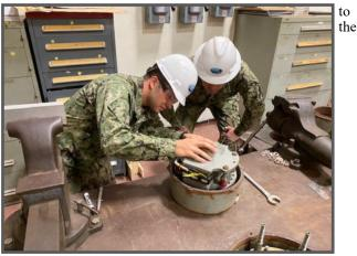
MM2(SW) Michael Bailey and MM2 James Lokey inspect a pad-eye electric motor brake for proper air gap clearance. The air gap needs to be close enough to catch once the brake is activated but not too close to cause dragging. This procedure is one of the more common jobs in the MARMC Outside Machine Shop. (Photo taken by MM2(SW) Jonathan Lepley.)
