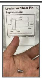
drawing of the shear pin laid out in metric measurements. Oddly enough, Monroe carries a copy of the drawing of this pin with both metric and Imperial (American standard) measurements in his notebook.
