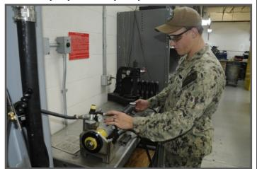
FC3 (SW) Christopher Bowdenwright testing recoil adapters on the shop's recoil test fixture.
